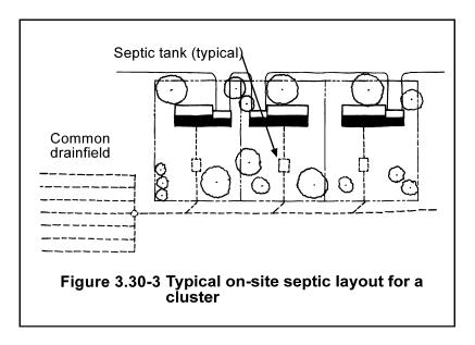
drainfields, package plants). These options can reduce infrastructure investment and allow placement of the systems in a way that will minimize adverse environmental impact. Figure 3.30-3 illustrates the use of a community septic drainfield as an alternative to individual systems.
